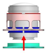
Insert the RC815-Z Zoom Gear on the plastic C-ring until it reaches the flange of the plastic C-ring.
