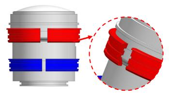
2. Insert the plastic C-ring for focus gear as shown and place it over the lens
