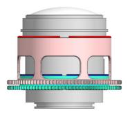
5. The tightness between the both gears and the lens can be adjusted by removing or adding rubber grips on either sides of the plastic C-ring, spare rubber grips are included in the package.
