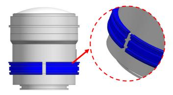
Insert the plastic C-ring for zoom gear as shown and place it over the lens
