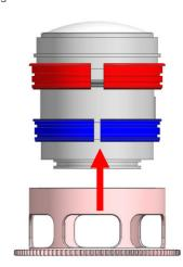
3. Insert the RC815-F Focus Gear on the plastic C-ring until it reaches the flange of the plastic C-ring.
